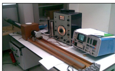
Figure 2 Sound absorption properties of small samples
