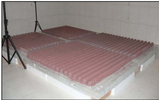
Fig. 3 Real scale test samples in the reverberation room
